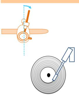
(N.B.) When setting the inside-force canceler, set with a zero balance without having a stlys pressure. Once the set-up of the anti-skating is completed, then adjust the stylus pressure with a stylus pressure gauge mounted on the round head enabling to match the stylus pressure of your cartridge.
